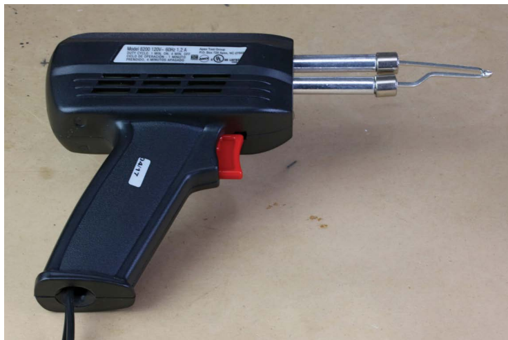
FIGURE 2-13: Pistol-grip soldering iron
