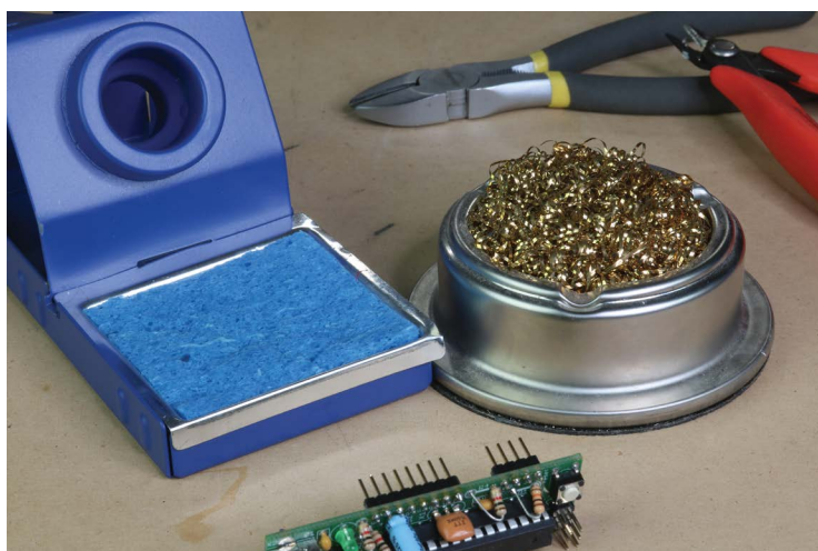
FIGURE 2-17: Two kinds of soldering iron sponges
