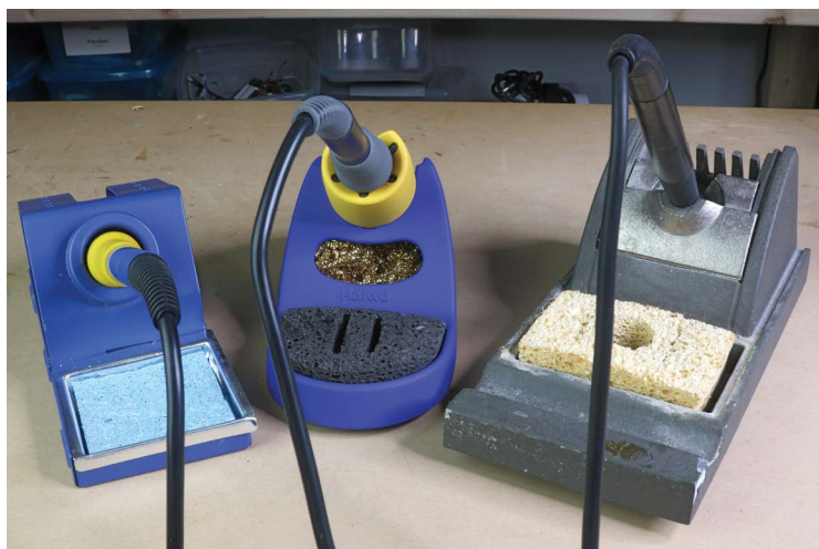
FIGURE 2-12: A variety of high-quality soldering iron stands
