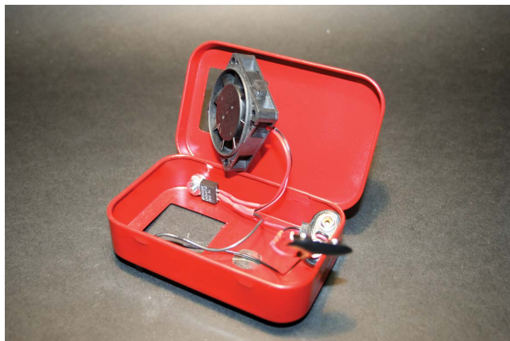
FIGURE 2-41: All the electrical components being installed
