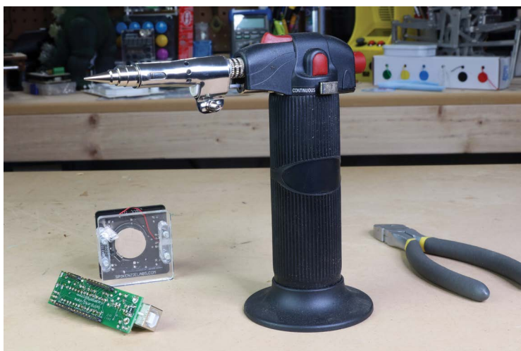
FIGURE 2-14: Gas-fueled soldering iron
