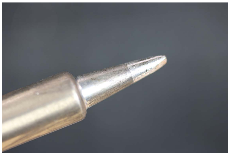
FIGURE 3-4: The tip after cleaning
