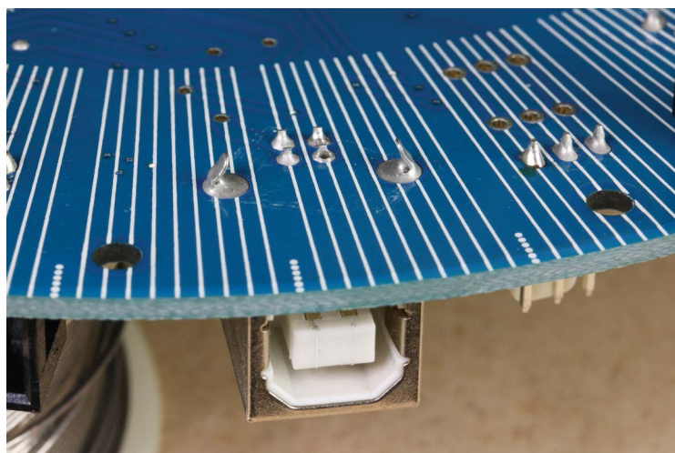
FIGURE 3-13: A USB connector with four leads and two lugs
