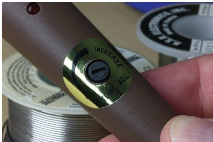
FIGURE 2-7: Temperature variation close-up shot
