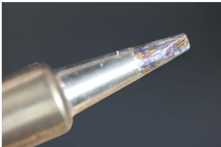
FIGURE 3-3: A dirty soldering iron
