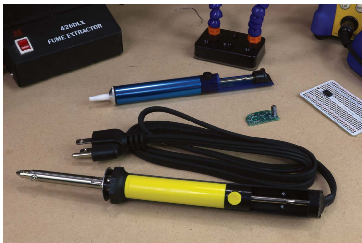
FIGURE 4-11: Electric solder sucker
