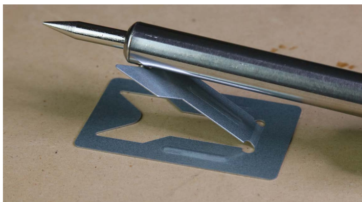
FIGURE 2-11: An example of a soldering iron stand that you should NOT use!
