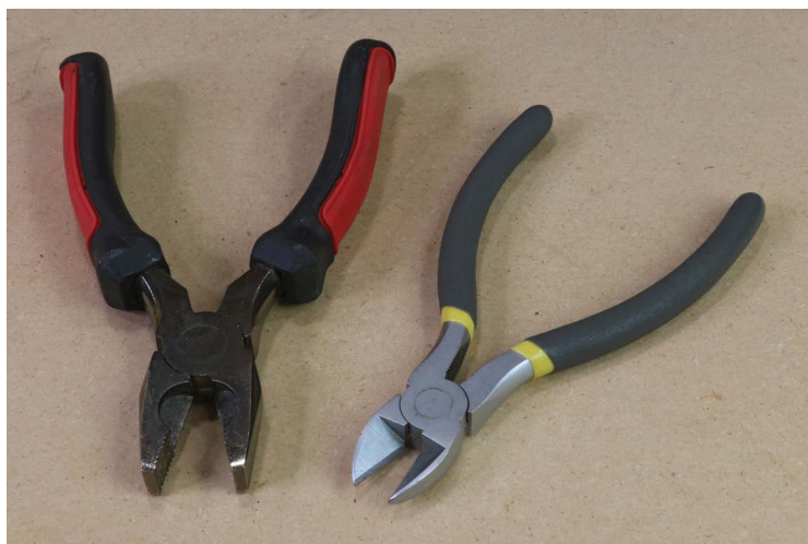
FIGURE 2-18: Two different kinds of wire-cutting pliers
