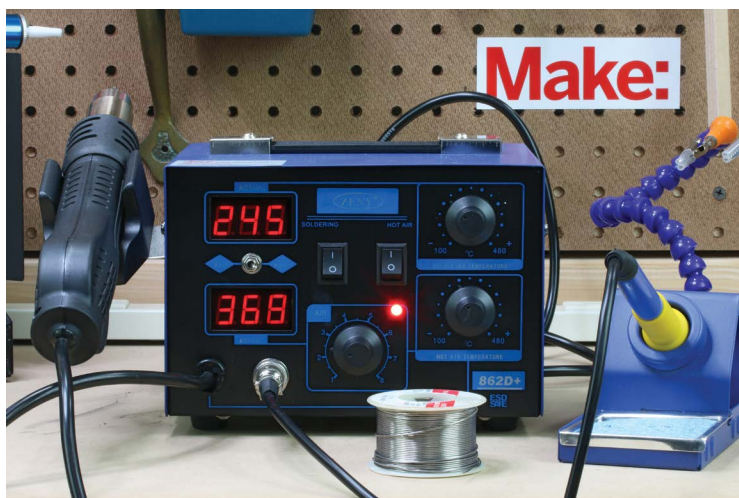
FIGURE 5-9: Hot air rework station
