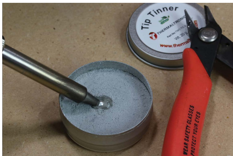
FIGURE 3-5: Using tip-tinning paste
